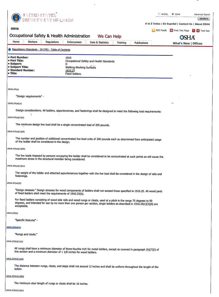
Rungs, cleats, and steps shall be ffee of splinters, sharp edges, burrs, or projections which may be a hazard.
